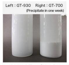
Dispersion stability of titanium oxide (The dispersion is stable over 3 months at 25°C)
